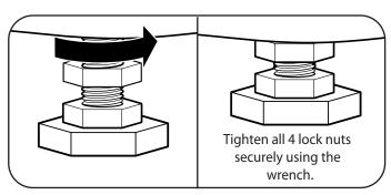
3. Once the washer is level from side to side and front to back, use the adjusting wrench to tighten all four lock nuts securely to prevent the legs from getting out of adjustment during operation. Make sure that all four leveling feet are in firm contact with the floor.
